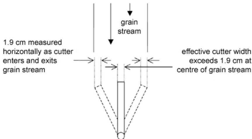
**Cutter opening requirement for arc-path cross-stream samplers.** The line drawing is showing the cutter opening measuring at least 1.9 cm (0.75 inches) as it enters the grain stream, when it is at the centre of the grain stream, and as it exits the grain stream.
