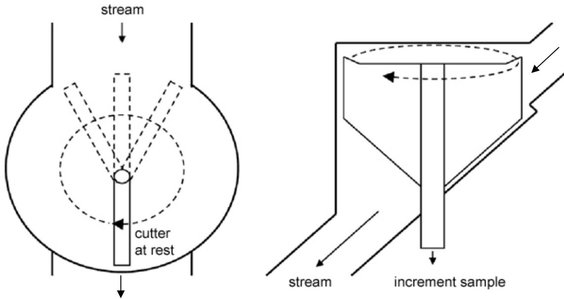
**Flowing stream.** The line drawing is showing a top view and a side view of the flowing stream type of arc-path cross-stream sampler. The diagram shows the direction of the grain stream, the sampler cutter trajectory, and the direction of the increment sample.
