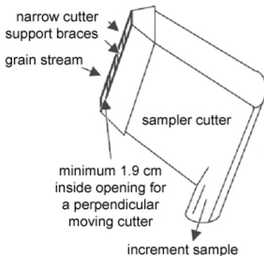
The line drawing is showing a sampler cutter in which the opening is reinforced with narrow support braces. The diagram shows the direction of grain stream and increment sample.
