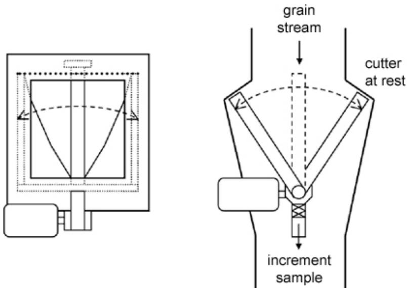
**Falling stream.** The line drawing is showing a top view and a side view of the falling stream type of arc-path cross-stream sampler. The diagram shows the direction of the grain stream, the sampler cutter trajectory, and the direction of the increment sample.
