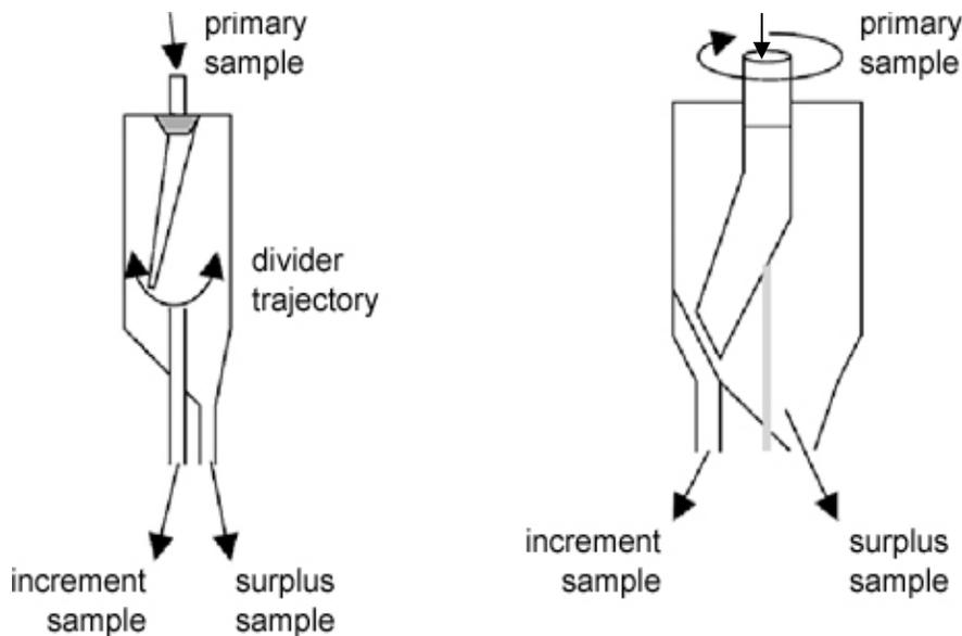
The line drawing is showing a swing arm divider and a rotary divider. In both diagrams the path of the increment sample and the path of the surplus sample are shown.
