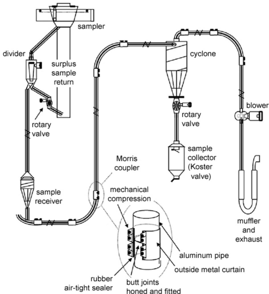
**Basic automatic sampling system configuration.** The line drawing is showing the path a sample takes from the sampler through to the sample collector (Koster valve). The diagram includes an expanded schematic of a Morris coupler. Morris couplers are used at various points along the delivery lines.
