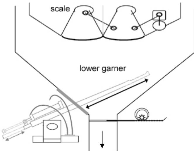
The line drawing shows a point type sampler. The sampling tube extends to at least 75% of the width of the grain stream.
