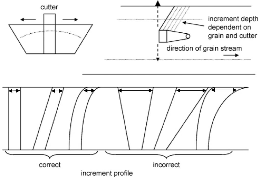
**Cross-stream sampler cutter path.** The line drawing is showing the requirements for sampling using a cross-stream sampler. The diagram shows the sampler cutter trajectory and direction, and illustrates both a correct sample increment and an incorrect sample increment. The diagram shows that the width of the increment must be the same, regardless of where it is taken in the grain flow.
